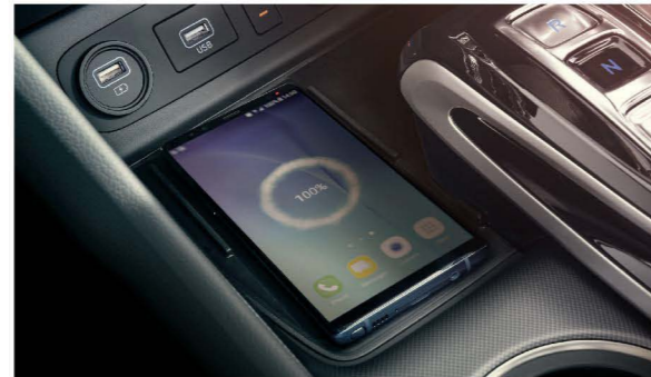
Wireless smartphone charging with temperature sensor and cooling function.
