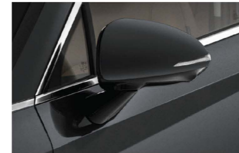
Side mirror with electric control & folding
